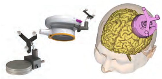
fUS tracking and custom fUS arms for large transducers
